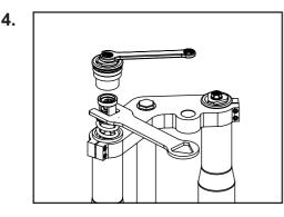
Remove the top cap nut assembly from the piston rod joiner using a 14mm spanner and the 17mm steel spanner provided -Tool No. 113-010-020.
