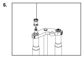
If a large amount of oil has been lost removing the spring it is necessary to check the oil level. To do this you will need to remove the spring preload spacer from under the main spring using a wire hook.
