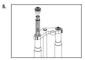
Remove the nylon spring pusher and the main spring slowly, keeping as much oil in the fork leg as possible.
