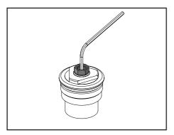
**Compression Damping:-** 3mm allen key in centre of the **BLACK** LEFT hand fork cap.
