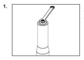
Remove all the preload from both forks using the 14mm hex in the centre of the top cap.
