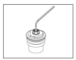
**Rebound Damping:-** 3mm allen key in centre of the **NATURAL** RIGHT hand fork cap.
