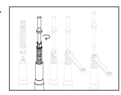
Using the pull up rod supplied - Tool No. 113-030-015 screw this onto the piston rod joiner.
