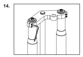
Tighten the upper fork clamp bolt to manufacturer's specification and adjust preload and damping settings to previous or recommended settings. (Located at the front of document)
