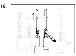
Pull the piston rod up and locate the 17mm steel spanner provided Tool No. 113-010-020 through the nylon spring pusher onto the 17mm hex on the piston rod joiner.
