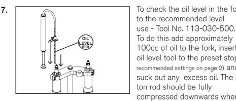
To do this add approximately 100cc of oil to the fork, insert the oil level tool to the preset stop (see recommended settings on page 2) and suck out any excess oil. The piston rod should be fully compressed downwards when performing this procedure.
