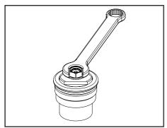
**Spring Preload:-** 14mm hex nut in centre of the fork caps. Spring preload has 18mm of adjustment, 1 turn on hex nut equals 1mm of preload on spring. Spring preload should be set from the fully open (anti-clockwise) position.
